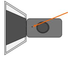
1. Switch the unit on by inserting the pin provided, into the hole in the base (you should hear an audible click) and the unit will commence flashing.
