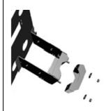
4. The TS2509 additional panel kit can now be positioned on the pole. The panel should face in the same direction as the panel attached to the beacon. Disconnect the nuts and washers from the bolts to detach the fixing bracket. Re-attach once the panel
