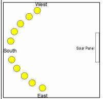
To position the beacon, please stand in the beacons intended location facing south (use the compass provided). Follow the arc of the sun, which travels east to west, to decide the least obstructed direction to position the solar panel.
