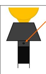
3. Drill two 4mm holes as a guide, into the pole, to line up with the mounting holes in the base of the Beacon. Use the 8mm socket and drill to fix the selftapping screws provided into the holes to secure the Beacon.
